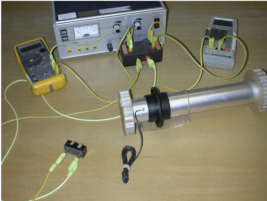
Photo no. 3: Measurements setup for ESD System 50 Flex-arm, test of base unit.
