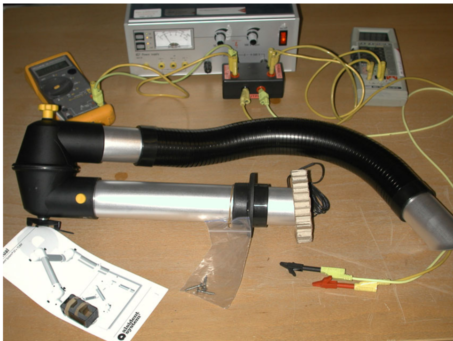
Photo no. 2: Measurements setup for ESD System 50 Flex-arm
